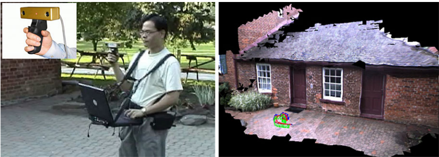
Fig. 2.20 The user points the stereo camera freely at the scene of interest ( left ) and the photo-realistic 3D model of the scene is generated ( right ). Figure adapted from [47]
