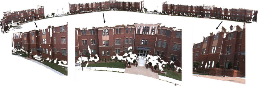
Fig. 2.19 An example of 3D modeling of urban scene from the Urbanscape project. Figure courtesy of [36]
