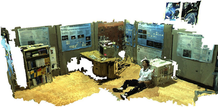
Fig. 2.23 3D model of a mock crime scene obtained with a hand-held stereo camera. Figure courtesy of [48]
