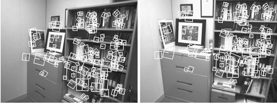
Fig. 2.12 Wide baseline matching between two images with SIFT. The size and orientation of the squares correspond to the scale and orientation of the matching SIFT features
