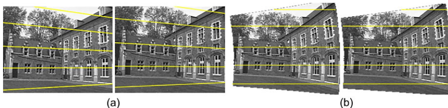
Fig. 2.10 An image pair before rectification (a) and after rectification (b). The overlay shows that the corresponding left and right features lie on the same image row after rectification. Figure courtesy of [43]
