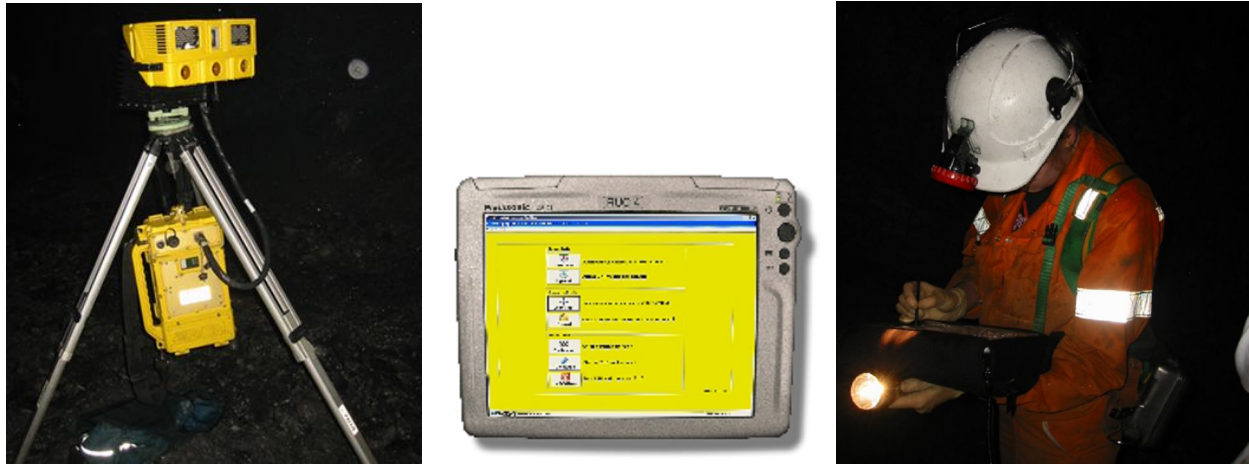
Figure 2 Motorized camera head on a tripod and Ruggedized Underground Computer hanging beneath the tripod (left). Hand-held wireless touch-screen (middle). Geotech annotating geological information onto a 3D model using the wireless touch-screen (right).
