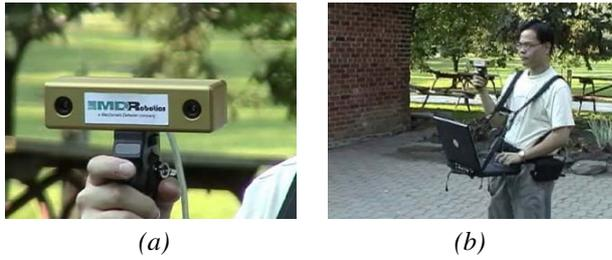
Figure 2. (a) *iSM* hand-held stereo camera. (b) *iSM* laptop carried by the user on a harness.
