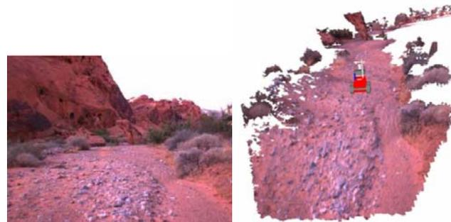
Figure 8 An image from a sequence taken by the MDA Autonomous Vehicle at a desert in Nevada (left) and the reconstructed 3D model with the vehicle model inserted for visualization (right).
