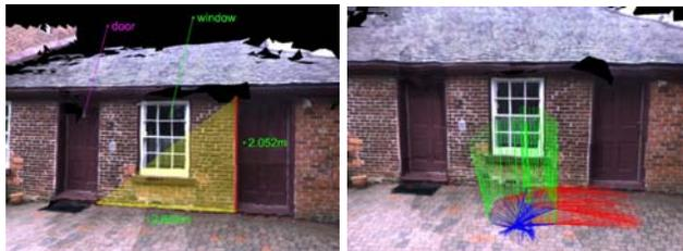
Figure 6 iSM visualization GUI showing the annotation and measurement (left) and the recovered camera trajectory (right)
