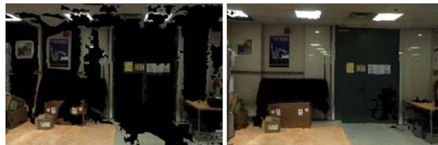
Figure 15 Screenshots of 3D model without (left) and with the pattern projector (right)
