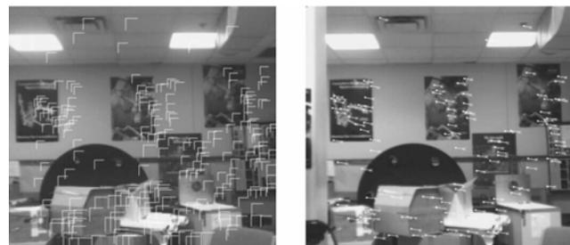
Figure 2 Stereo matched SIFT features (left) and SIFT features that are matched to the database (right)
