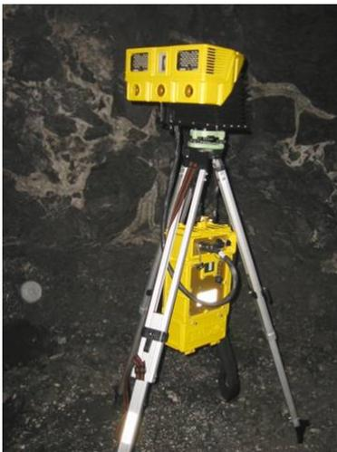
Figure 11 instant Mine Modeler – a motorized version of iSM
