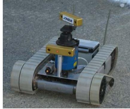
Figure 16 A proof-of-concept iSM 3D modeling payload mounted on the iRobot Wayfarer PackBot. The payload consists of a stereo camera (with the MDA logo) and a compact laptop at the back.
