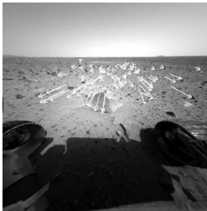
Figure 5: Temporal matching of SIFT features between frames
