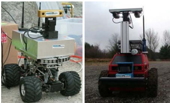
Figure 7: (Left) Custom rover with Bumblebee stereo camera. (Right) ATRVJr rover with custom stereo camera.
