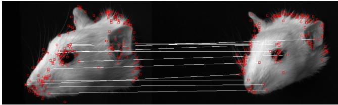
**Fig. 2.** Example of SIFT features (red) and matches (white lines) for a pair of images of a rat head.
