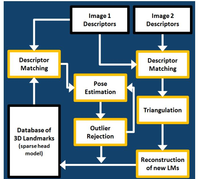
**Fig. 3.** Landmark (LM) generation and pose estimation. Feature (descriptor) matching between a pair of images enabled 3D LM to be reconstructed using triangulation. Matching between an image and the LM database enabled pose estimation (see Fig. 4). Once pose had been estimated, new LMs were added to the database consistent with the initial (frame 1) pose.
