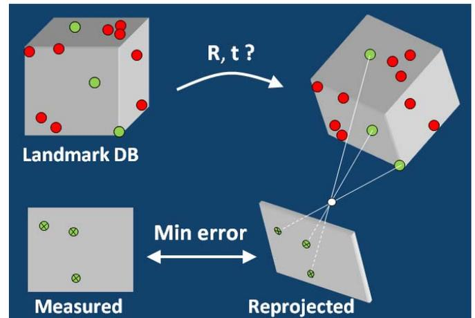
**Fig. 4.** Pose estimation. Once matches (here shown in green) had been found between a camera image and the descriptors in the database, pose estimation was the task of determining the rotation,  $\mathbf{R}$ , and translation,  $\mathbf{t}$ , minimizing the reprojection error. Instead of determining the pose directly, a correction to the previous pose was determined (see [3] for details).
