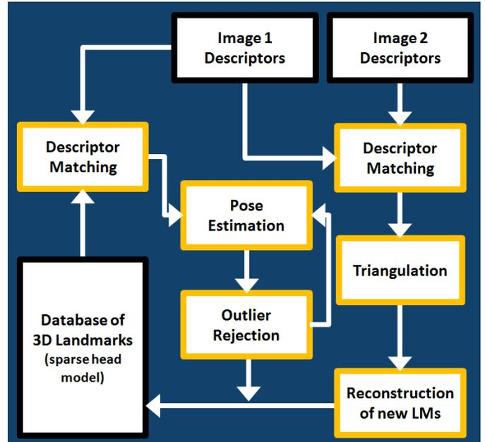
**Fig. 3.** Landmark (LM) generation and pose estimation. Feature (descriptor) matching between a pair of images enabled 3D LMs to be reconstructed using triangulation. Matching between an image and the LM database enabled pose estimation (see Fig. 4). Once pose had been estimated, new LMs were added to the database consistent with the initial (frame 1) pose.
