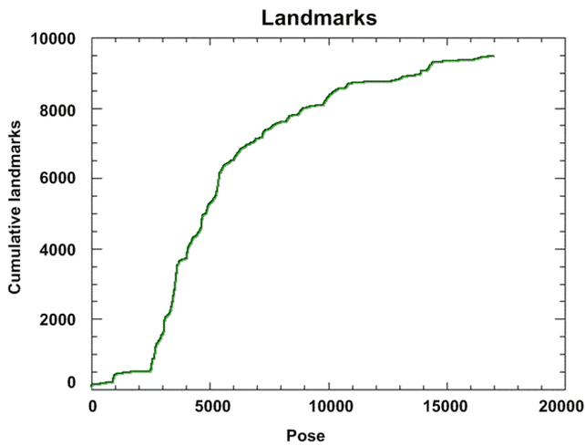
**Fig. 6.** Cumulative number of 3D head landmarks as a function of pose number.
