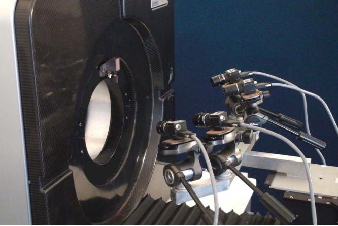
**Fig. 1.** Setup for markerless motion tracking. The four cameras were mounted to the microPET via an aluminium frame.
