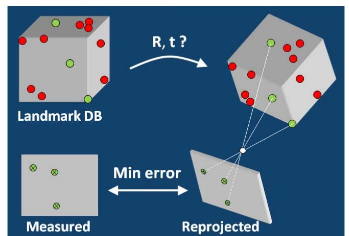
**Fig. 4.** Pose estimation. Once matches (here shown in green) had been found between a camera image and the descriptors in the database, pose estimation was the task of determining the rotation,  $R$ , and translation,  $t$ , minimizing the reprojection error. Instead of determining the pose directly, a correction to the previous pose was determined (see [3] for details).
