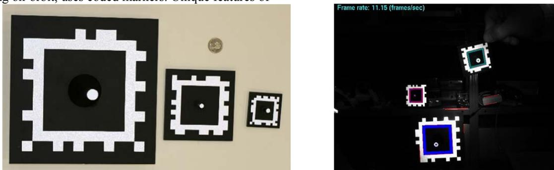
Figure 1. SVMS markers on a planar surface (left) and detected in a scene (right)
