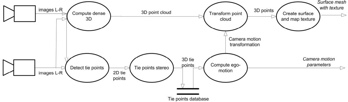
Figure 6 iSM system architecture
