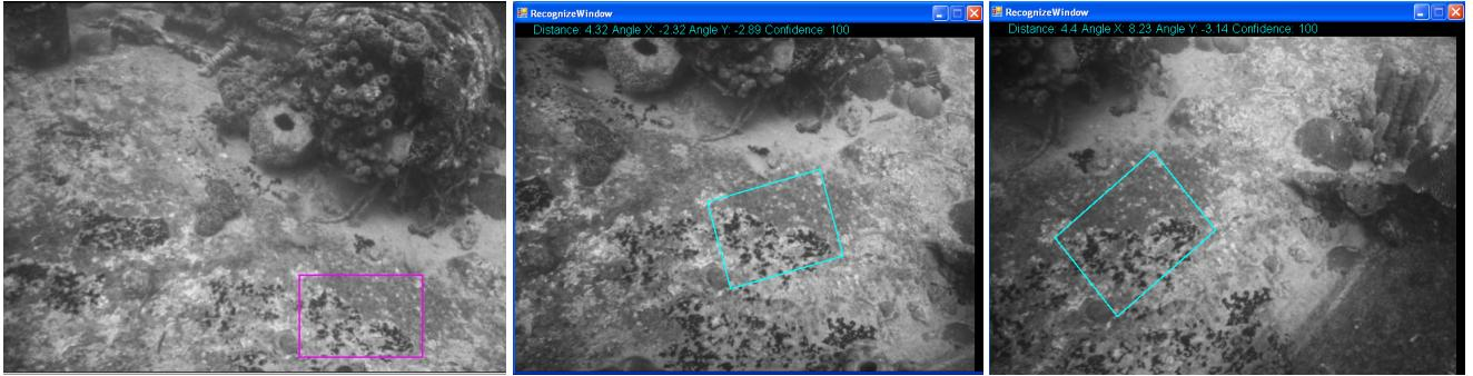
Figure 4 An object of interest is selected in the first image (purple rectangle in the left image) and automatically tracked in the subsequent images (middle and right)
