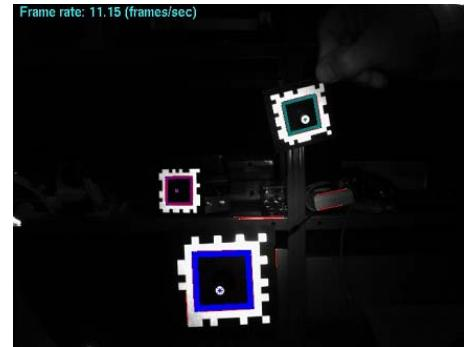
The SVMS vision system uses calibrated cameras and provides complete information on the relative target location (position and orientation – 6 degrees of freedom). Fig.2 shows images of the SVMS target detected in a hand held camera sequence, captured underwater in a swimming pool: blue overlays on the target indicate correct detection (marker is black and white) and the numbers on the top of
