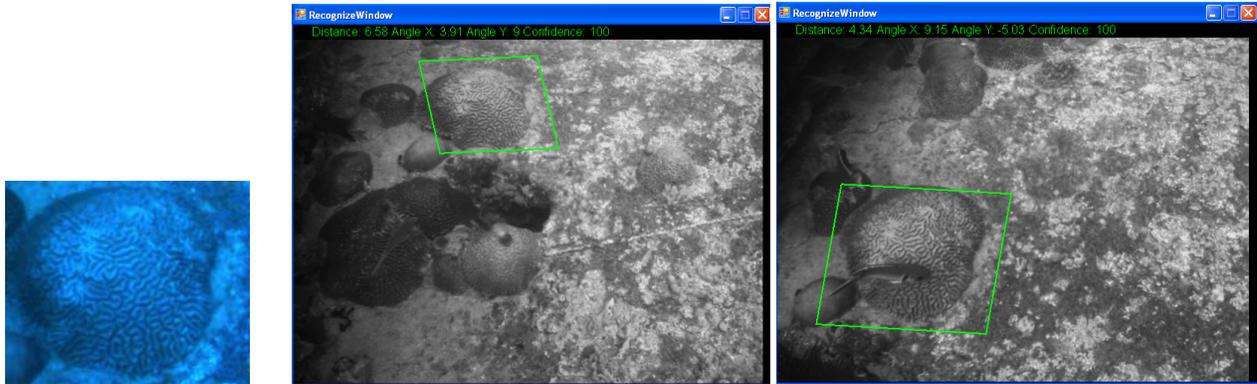
Figure 5 A coral reef is selected as target a(left) and automatically detected and tracked in the image sequence (middle and right).
