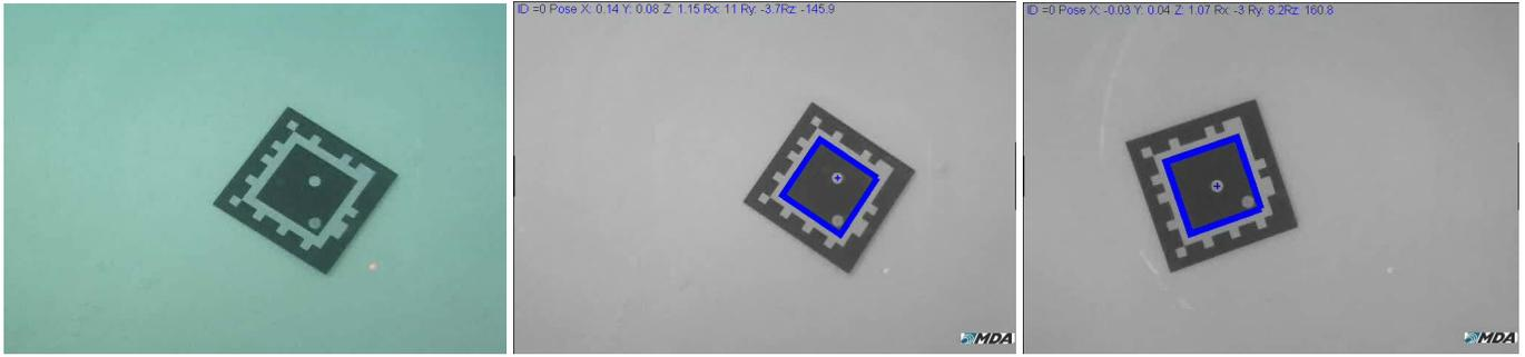
Figure 2 An input image from an underwater image sequence (left) and the SVMS target detected with computed pose (middle and right)
