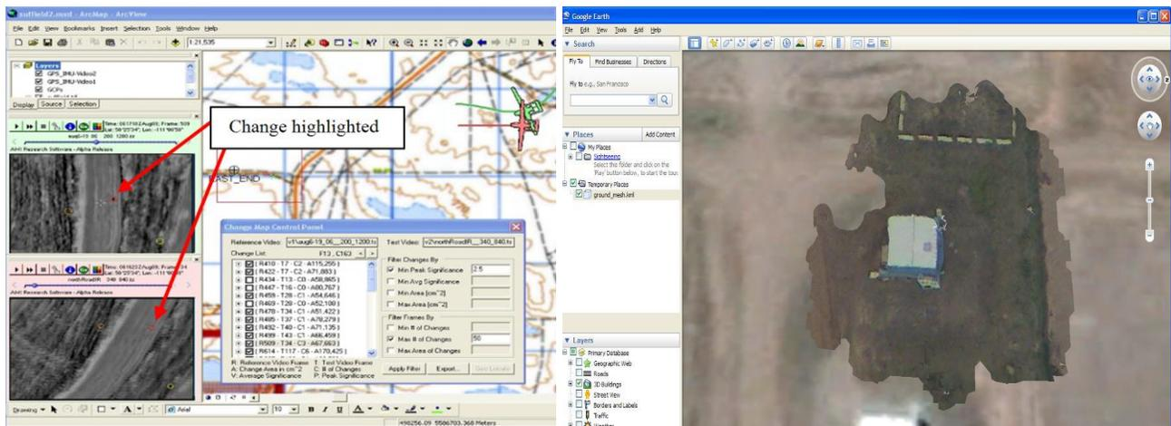
Figure 5 AMIE Change Detection Tool (left) and 3D Model Generated by AMIE 3D Reconstruction Tool (right)
