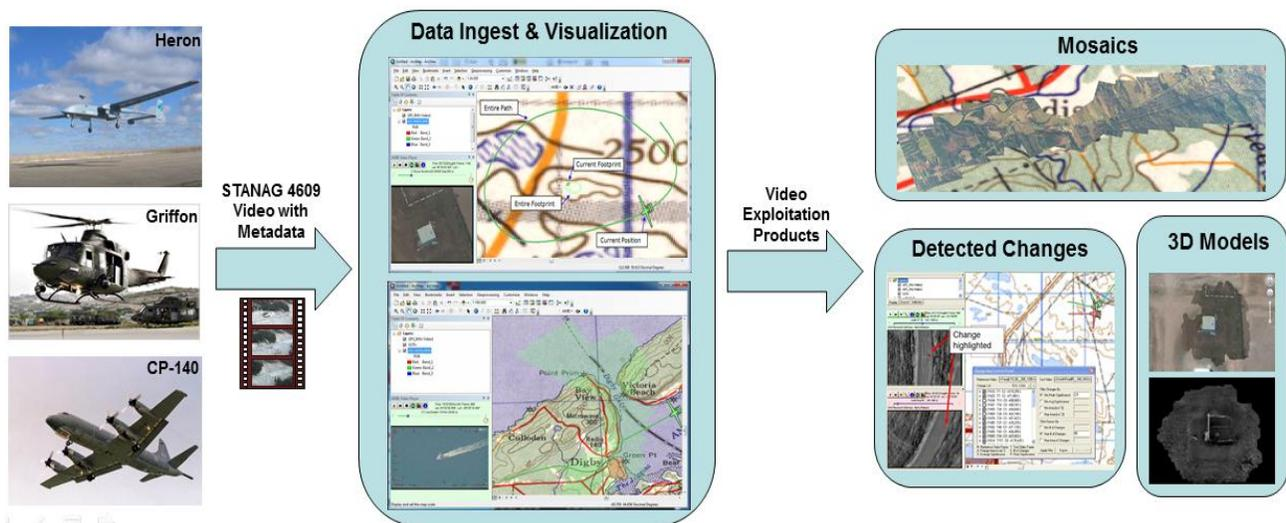
Figure 1 High-level Functionalities of the AMIE System (Image Source: DND, Map Source: DMAAC)
