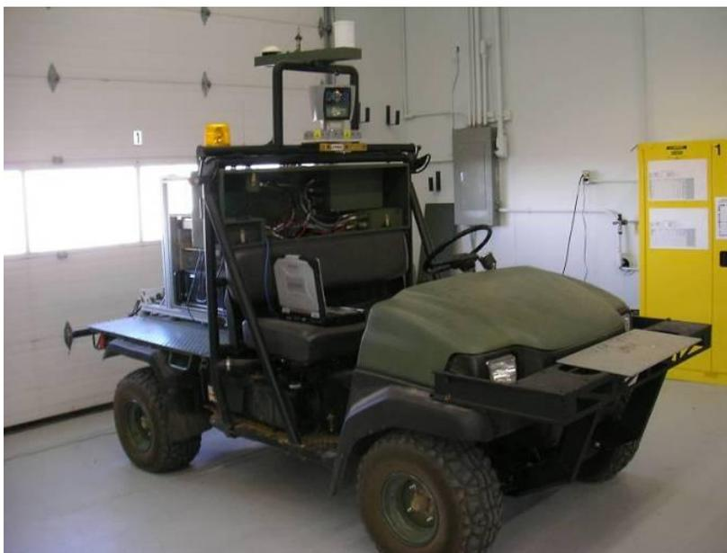
Figure 3. Research platform used to conduct the tests. The Velodyne lidar housed on top of the vehicle was used for all tests.
