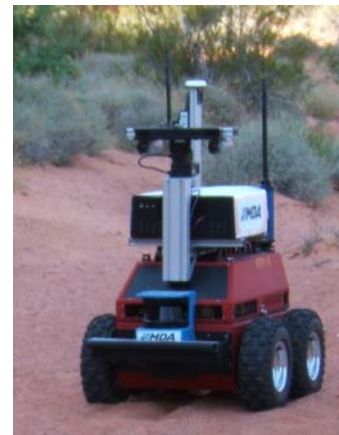
Figure 7 Vehicle mounted stereo cameras and vision system
