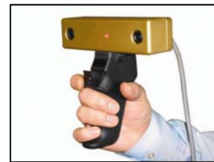
Figure 2 Hand held instant Scene Modeler (iSM)
